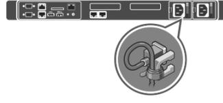
**4** Loop and secure the power cable by using the retention strap.
